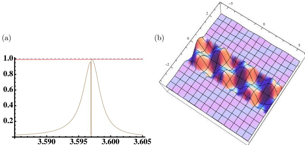
**Figure 5.** Normalised transmitted energy versus spectral parameter  $\beta$  for a triplet of rigid pins with angle of incidence  $\theta_i = 0.481273$  and shift of the central grating  $\xi = 0.012$  (b) Field plots for the example illustrated in (a).
