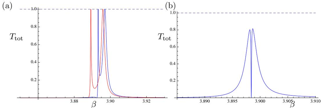
**Figure 2.** Total transmittance  $T_{\text{tot}}$  as a function of  $\beta$  for a triplet with a shifted central grating of finite radius inclusions with  $a = 0.0035d$ , and an outer pair of gratings of inclusions of radius  $a = 0.01d$ ,  $\theta_i = 26^\circ$ . Data used: (a)  $\xi = 0.4d$  (red curve),  $\xi = 0.42d$  (blue curve). (b)  $\xi = 0.45556d$ .
