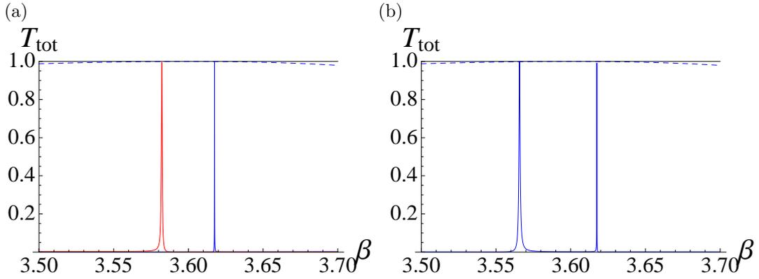
**Figure 6.** Normalised transmitted energy versus spectral parameter  $\beta$  for  $\theta_i = 30^\circ$  for (a) a pair of rigid pin gratings with  $\eta = d$  (red curve) and  $\eta = 2d$  (blue curve). (b) a triplet of rigid pin gratings.
