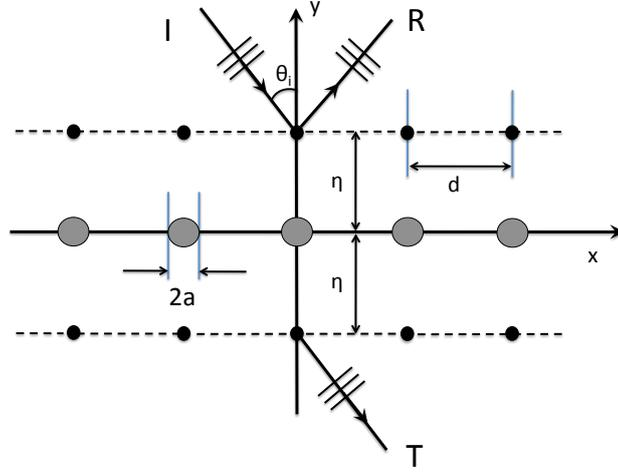
**Figure 1.** Stack of gratings consisting of an outer pair of rigid pins and a central grating of finite nonzero inclusions with radius  $a$  and period  $d$ . The relative grating separation between consecutive gratings is denoted by  $\eta$ .
