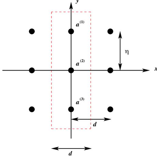
**Figure 3.** Elementary cell for the waveguide consisting of a triplet of unshifted rigid pin gratings.
