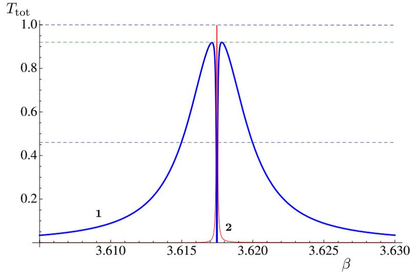
**Figure 7.** EDIT effect for a triplet of rigid pin gratings with the central grating shifted by  $\xi = 0.25200d$  for the angle of incidence  $\theta_i = 30^\circ$ . Total transmittance  $T_{\text{tot}}$  (curve 1) as a function of  $\beta$  for the triplet. Curve 2 represents the total transmittance for the outer pair of gratings.
