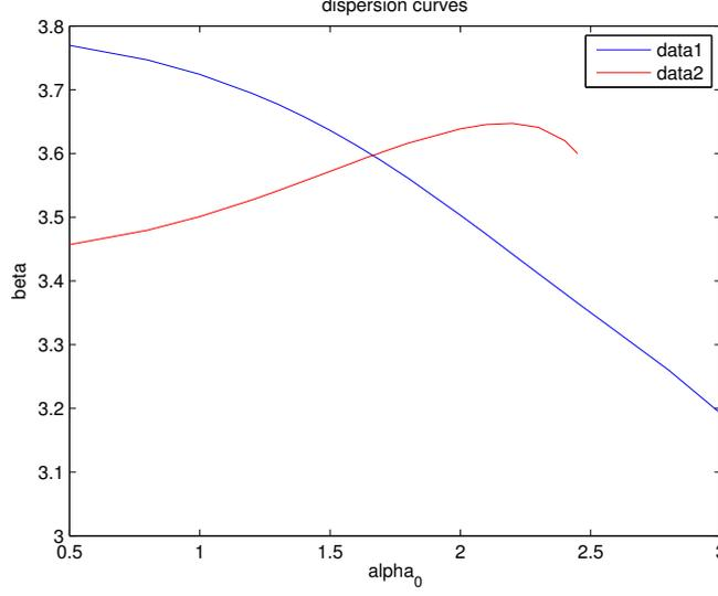
**Figure 4.** Dispersion diagram for a waveguide consisting of an unshifted triplet with the horizontal axis representing  $\alpha_0$  in the range  $0 \leq \alpha_0 \leq \pi$ , and  $\beta$  on the vertical axis in the range  $2 \leq \beta \leq 4$ . Produced using *Matlab*. The red curve represents the odd modes, and the blue curve, the even modes.
